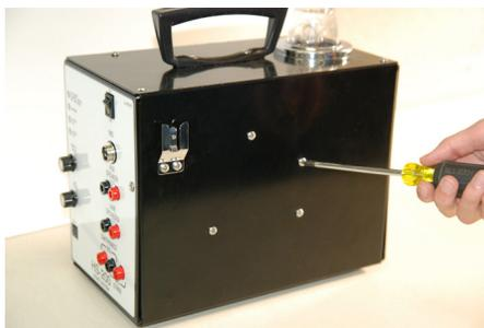
Figure 14: Remove Screws
