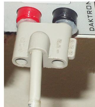
**Figure 10:** Insert GND Side to Black Female Jack
