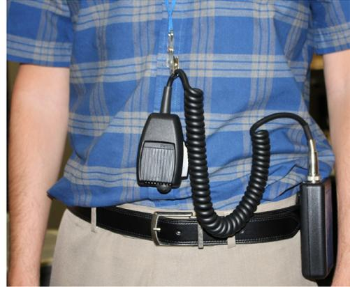
**Figure 17:** Wireless Unit & Microphone
